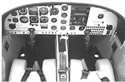
**The Micco SP20's standard equipment includes fuel dual controls with single throttle on a console between pilots.**
