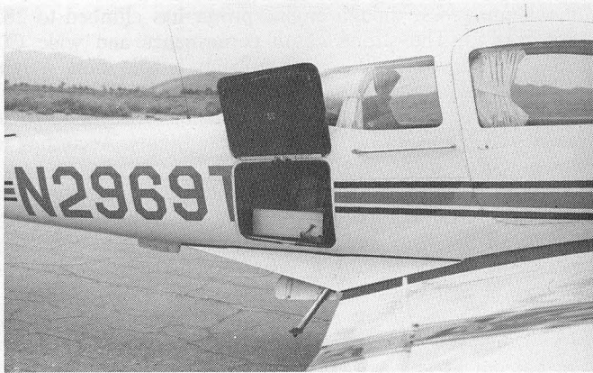
Though a tight, trim airplane in most respects, the Commander 200 has reasonable access to necessary areas. At left, owner Don Coniglio opens the door right over the oil dipstick. Above, the baggage hatch is just aft of the wing where it can be easily loaded or unloaded. Below, the single passenger door is wide enough for easy entry into the rear seats. Note towel rack assist handle.
