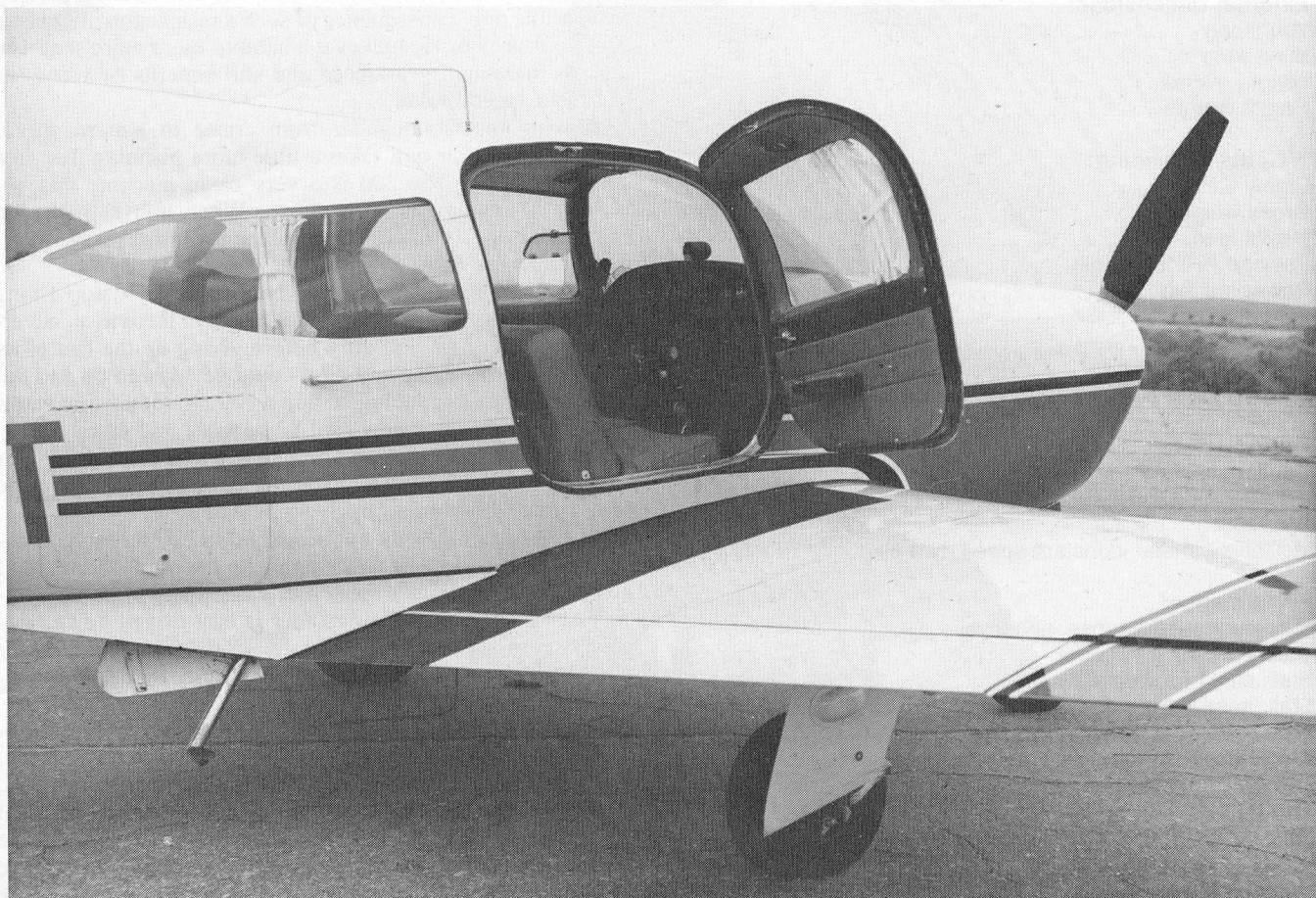
Though a tight, trim airplane in most respects, the Commander 200 has reasonable access to necessary areas. At left, owner Don Coniglio opens the door right over the oil dipstick. Above, the baggage hatch is just aft of the wing where it can be easily loaded or unloaded. Below, the single passenger door is wide enough for easy entry into the rear seats. Note towel rack assist handle.
