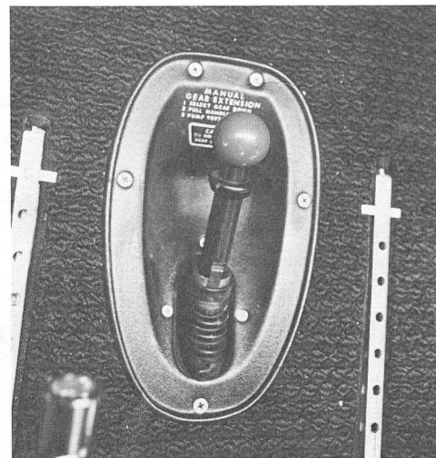
Between the front seats: an emergency gear extension pump handle. Both gear and flaps are hydraulic on the Meyers, and can be operated manually.
