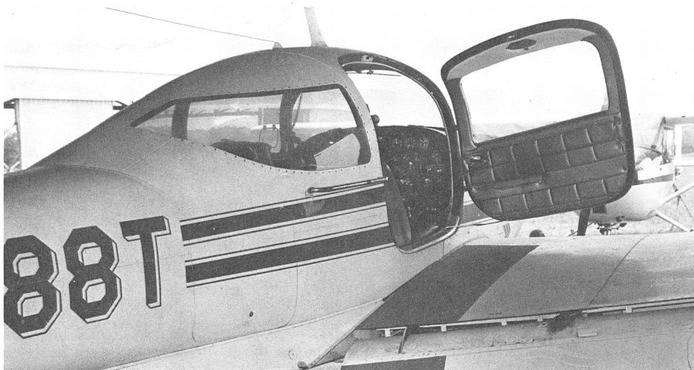
Massive bar alongside the door eases entry and typifies what operators characterize as a quality of being "overbuilt."
