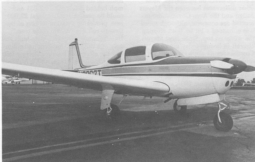
A generally slick aerodynamic package, despite the blunt nose, affords the Meyers its speed. Owners like to boast that the nosewheel is so well engineered it doesn't need a shimmy damper. Hidden beneath the smooth curves is a massive tubular framework that comprises the fuselage and cabin and the wing out to the landing gear.
