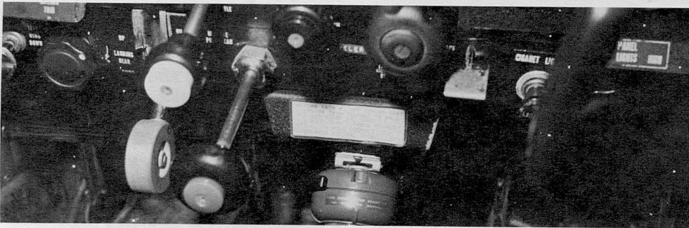
The aircraft has the luxury of both aileron and pitch trim. The unorthodox pitch trim is the knurled vernier knob above the mike; aileron trim is located at the left of the white-tipped throttle control. Mixture is below and between throttle and prop.
