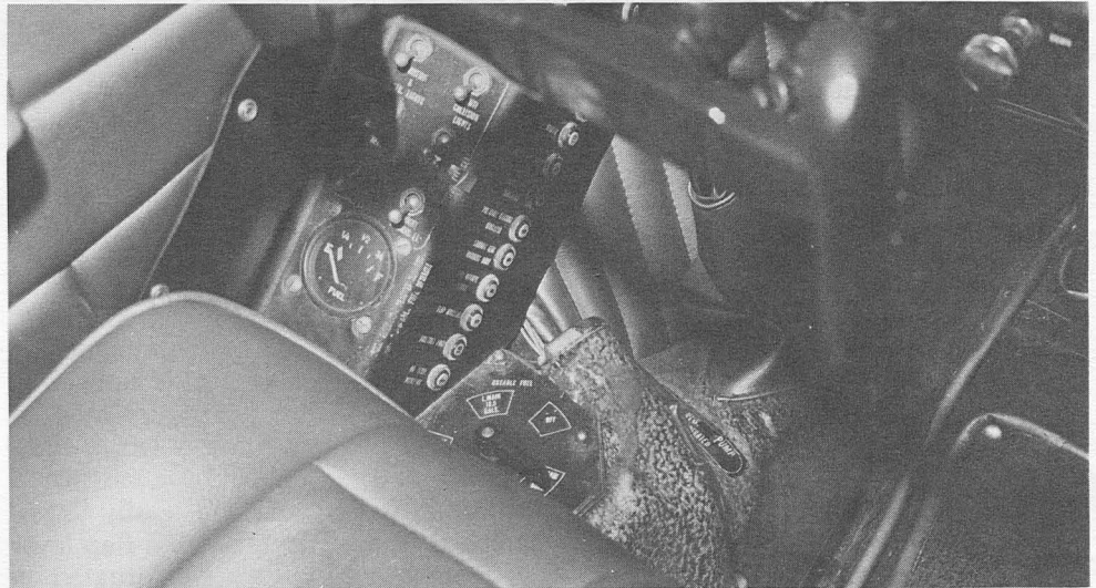
Fuel management calls for switching to four separate tanks with the lever at the left of the pilot's leg. Fuel gauge shows only the fuel in the tank selected.
