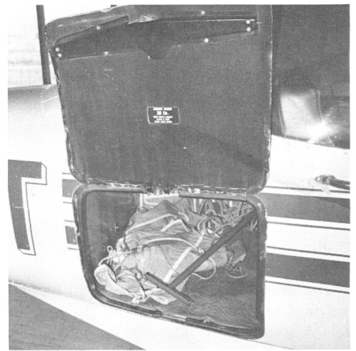
Baggage compartment holds a respectable 200 pounds structurally.
