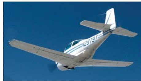
Viewed from below, this Meyers 200 shows off its (for the time) industry-leading features: tapered wings, fully enclosed landing gear and trailing-edge belly strakes. The only airframe ADs should have been complied with long ago.
