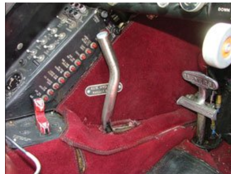
At the pilot's left knee are numerous switches and circuit breakers, along with the auxiliary hydraulic system's pump handle.
