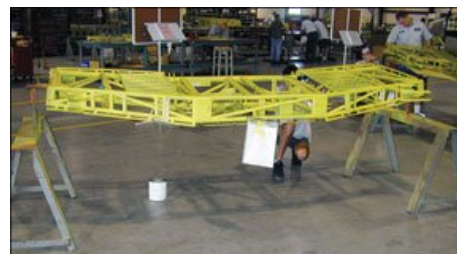
This wing center section for the Micco SP26—a modernized Meyers 145 that has an on-again/off-again story of its own—
